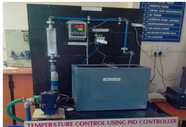
Figure 2: Temperature Control Loop
